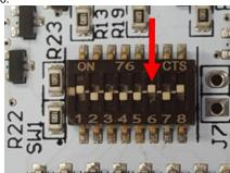
**NOTE:** For the Dip Switch setting to take effect the power and battery will need to be disconnected and reconnected.
