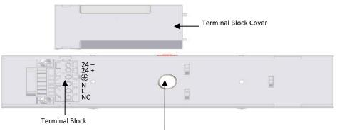
Cable Entry Point – Inside of bracket for ceiling mount, 20mm diameter, located in centre of bracket. Bracket show with the terminal block cover removed.
